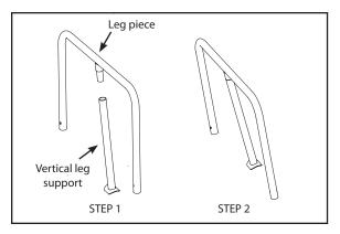
Figure 4-A: Assembling the leg pieces
