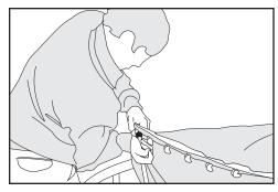
Figure 3: Preferred rod bending technique
