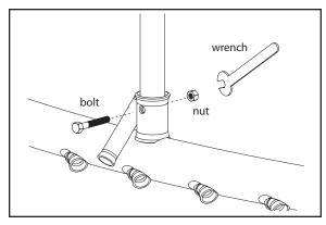
Figure 5: Fastening the legs to the frame
