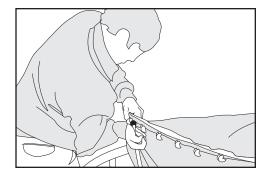
Figure 13-B: Preferred rod bending technique
