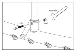
Figure 3: Fastening the legs to the frame
