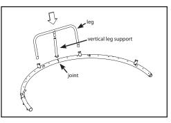
Figure 2-A: Inserting a leg piece and vertical support
