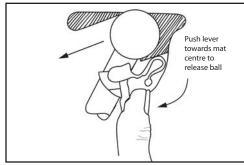
Figure 1: The release clip on the mat fitting
