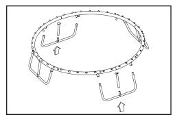
Figure 5: Attaching the final legs and vertical supports
