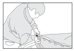
Figure 12-B: Preferred rod bending technique
