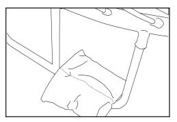
Figure 21-C: Placing the sandbag over the leg
