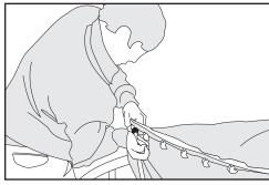
Figure 3: Preferred rod bending technique
