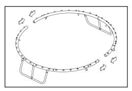
Figure 4: Connecting the frame sections
