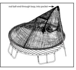
Figure 17: Inserting an elcosure rod into a pocket
