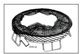
Figure 15: Sliding the net up the rods
