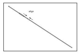
Figure 16-B: Aligning rod parts at the joint
