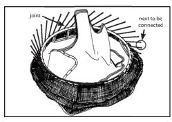
Figure 11-A: Attaching the mat to the rods
