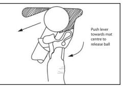
Figure 13-B: The release clip on the mat fitting
