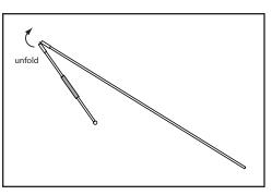
Figure 16-A: Straightening an enclosure rod
